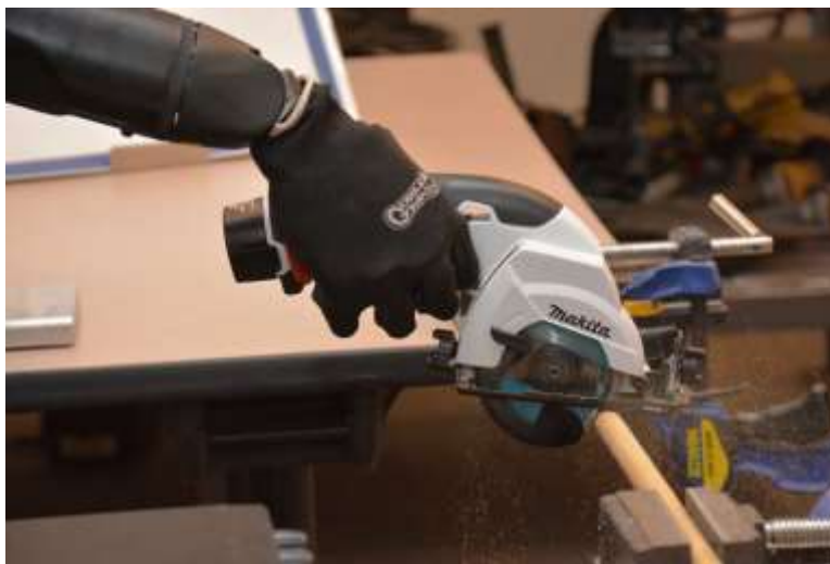
Figure 9: MPL cutting through dowel with hand saw
